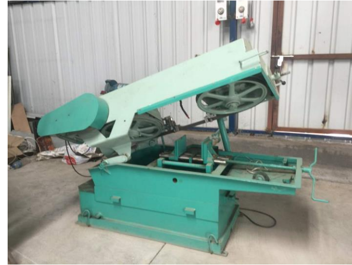
Band-saw cutting : 200mm ; 8 inch
