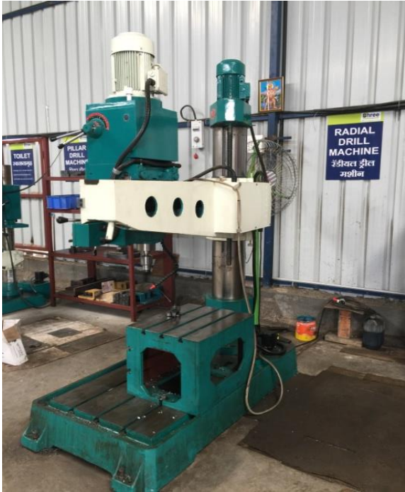
Radial Drill : 45mm ; arm 1 m
